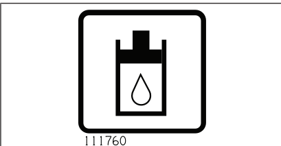
Hydraulic oil reservoir fill
